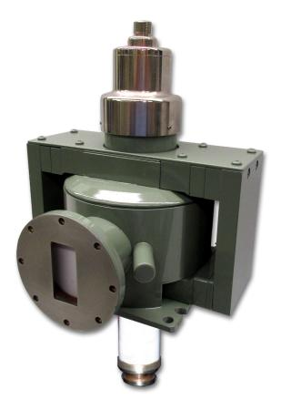
The VMC1891B is a coaxial magnetron that delivers high peak and average RF power for use in weather radar transmitters.
